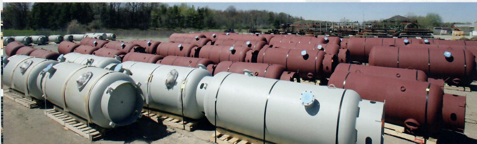
Industrial ASME air receivers
