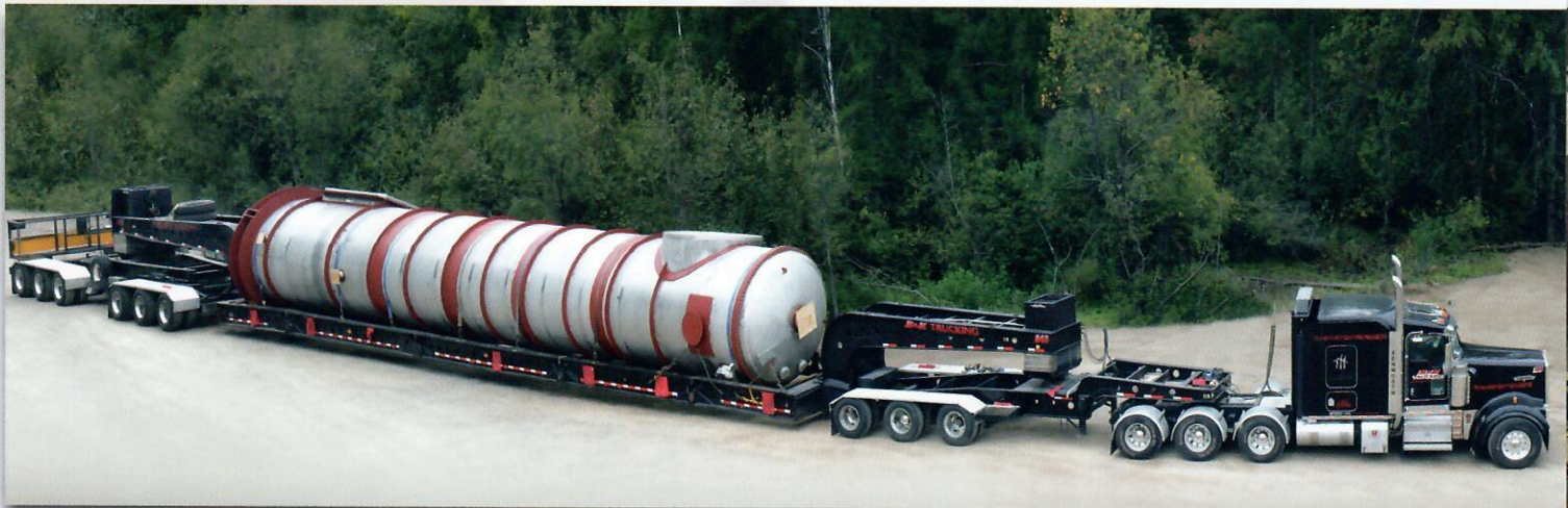
130,000 lb Shell and tube heat exchanger
