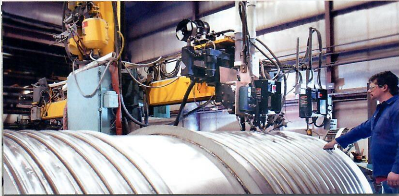
Full penetration half pipe – automated welding
