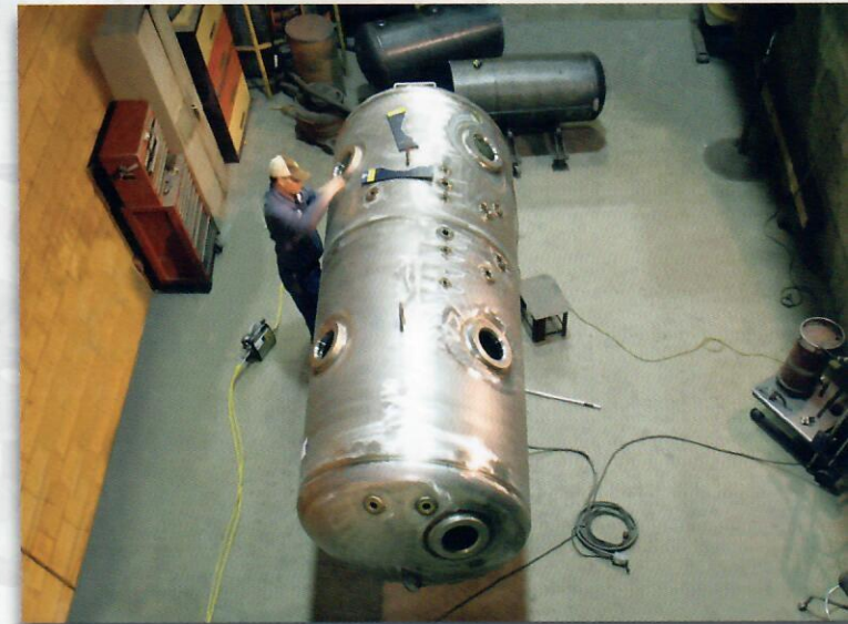
In house x-ray testing chamber and equipment
